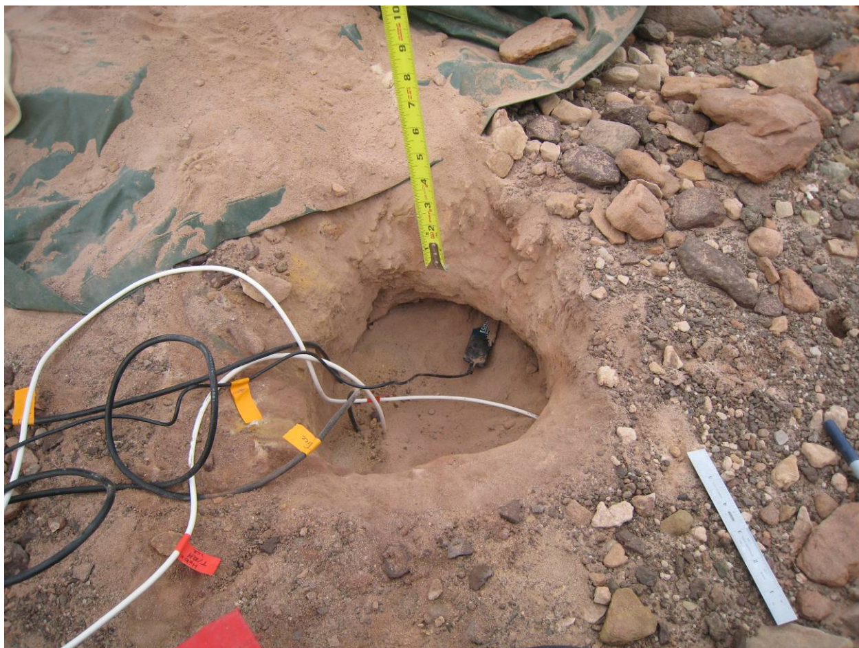
IMG_3595: The lowest level of instruments were already inserted (in the ice-cemented ground and at the ice-cemented ground boundary) and the hole partially filled on. This is the second layer of instruments at ~20 cm. The Echo is inserted in this image, as well as the 20 cm T/RH Hobo. The metal ruler on the right is 15 cm
