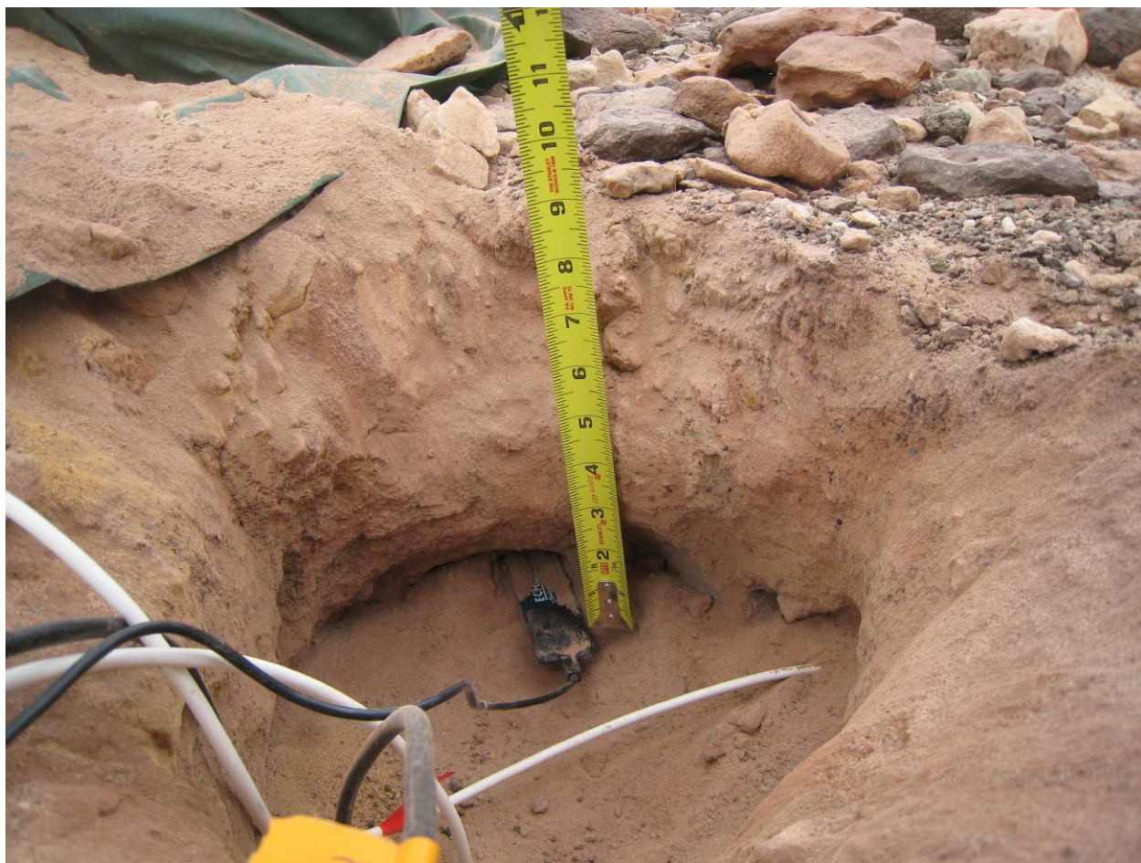
IMG_3596: Depth to the Echo sensor: 23 cm (9 inches). The regolith was pretty loose.
